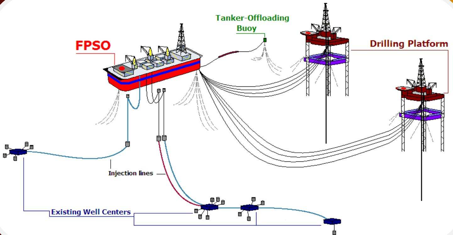
A floating production, storage and offloading (FPSO) unit is a floating vessel used by the offshore oil and gas industry for the processing of hydrocarbons and for storage of oil.
